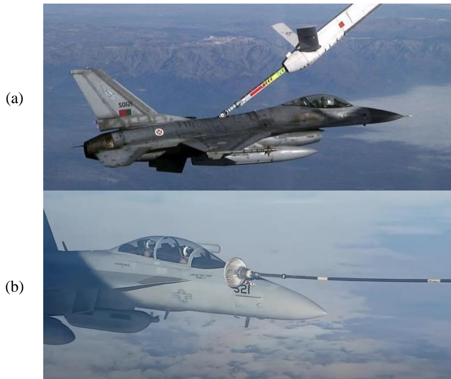
Figure 1.1: AAR systems: (a) flying boom [1], (b) probe-drogue [2].
